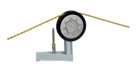
Pully complete with Scaffold Clamp. Complete with Short Frame block.
