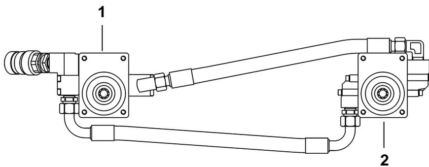
Fig. 1-9 Drive motor unit
