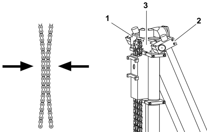
Fig. 6-3 Tensioning chain
