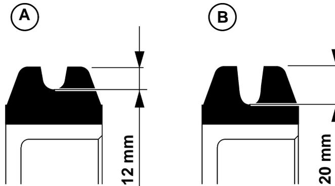
Fig. 6-1 Drive pulley bandage
