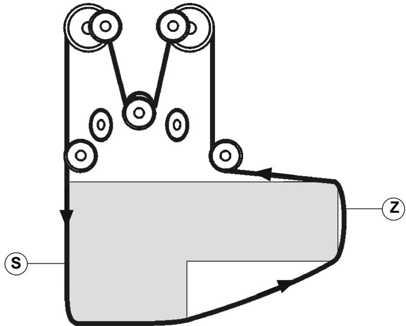
Fig. 5-3 Cutting direction
